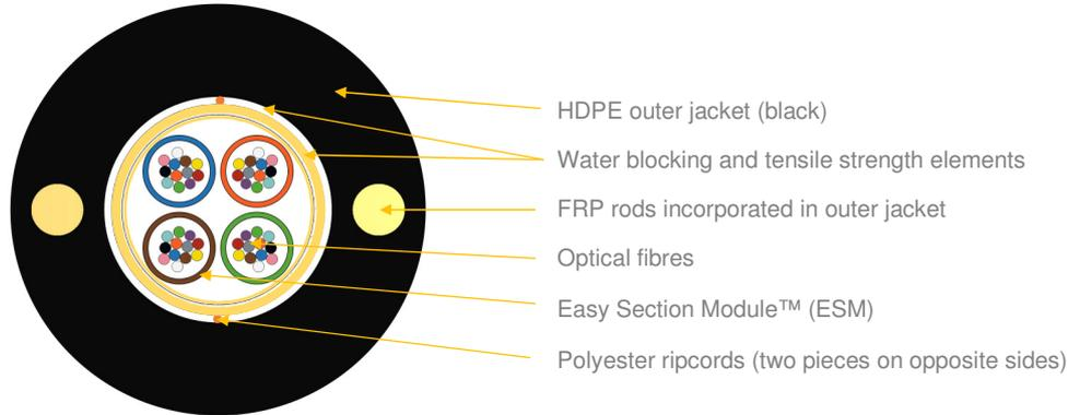
\*schematic drawing of 48F configuration, not to scale
