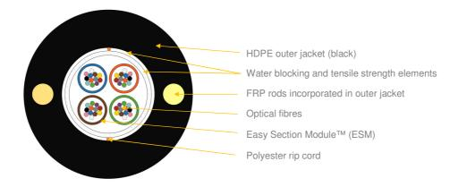
\*schematic drawing of 48F configuration, not to scale
