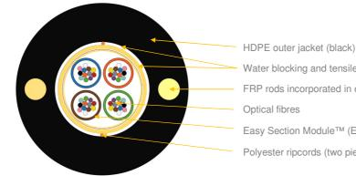
Water blocking and tensile strength elements
