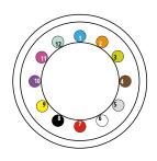
n 24-fiber tube construction colors will be repeated to facillitate identification, fibers 13-24 will have rings every 25 cm
